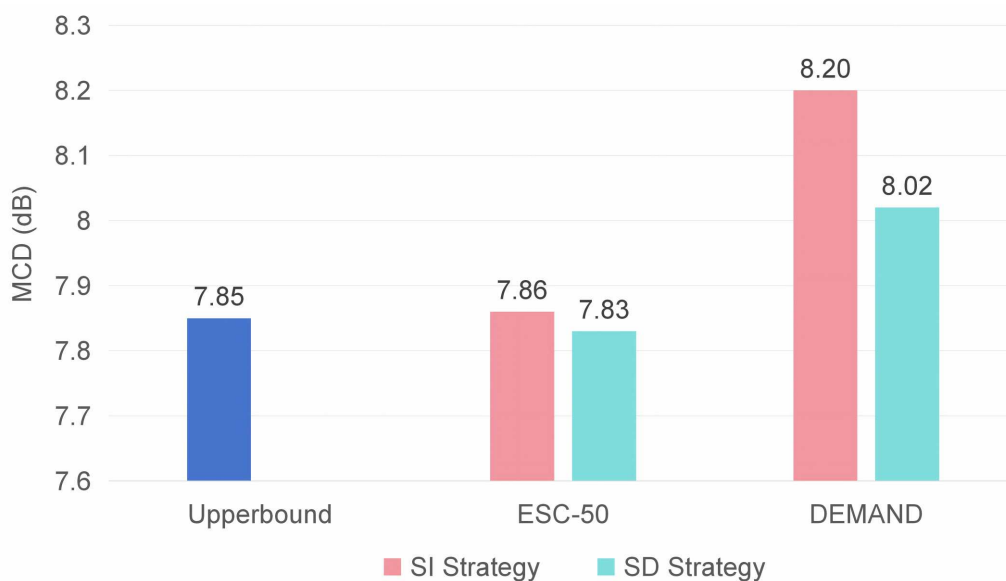
Figure 5.2: MCD results for N2N trained on the original noisy datasets using SI and SD noise sampling strategies.
