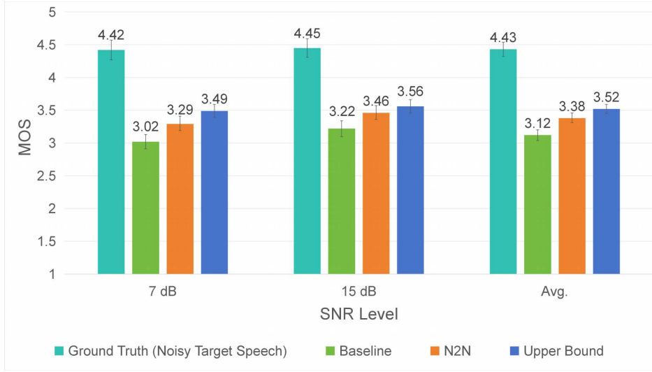
Figure 3.6: MOS results with 95% confidence intervals for Upper Bound, Baseline, and N2N. Ground Truth refers to the original noisy speech from the target speaker.
