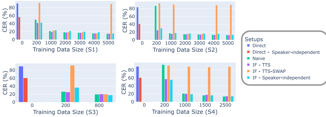
Figure 3.7: Character error rate (CER) of the different developed ASR systems for all speakers (S1, S2, S3, and S4). The x-axis indicates the amount of data used in the training and development sets.
